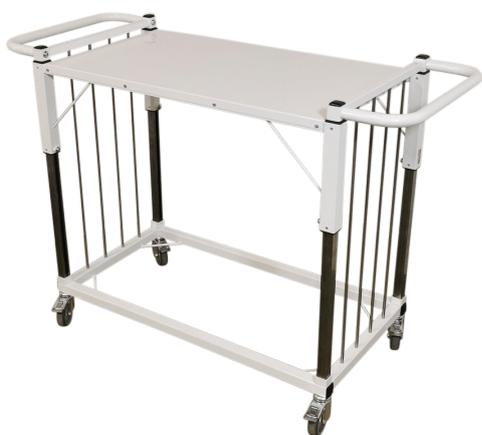
Ergonomic picking trolley with springs - 850x450x800 mm, where the table top automatically adjusts to the weight. At 30 kg, the table bottoms out and can carry up to 100 kg. Equipped with Ø75 wheels for stable and easy maneuvering in warehouse and production.
